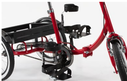
846 Ankle support with calf adjustment (for use with the 841 pedal cage).
