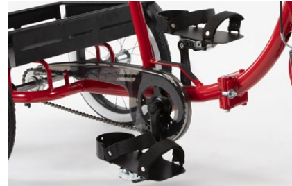
841 Pedal cage with foot imprint and fastening strap.
